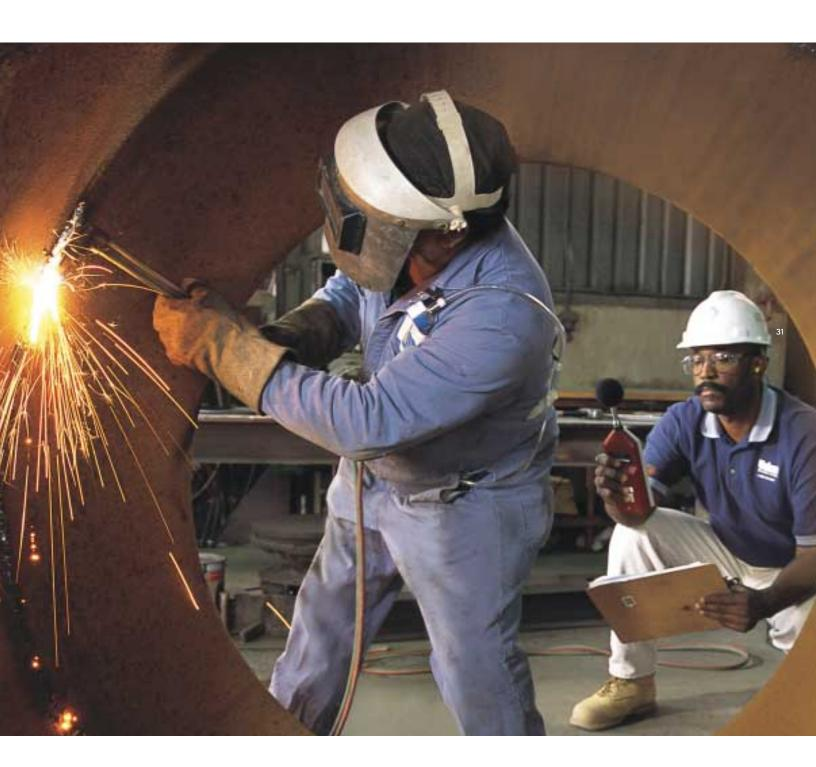
Trained sampling technicians use sound-level meters to make sure we meet both our own noise exposure standards and those set by regulatory agencies. We monitor noise generated by equipment and activities (such as welding) at all our facilities. Maintaining acceptable levels is important to protect both our workers and our neighbors.
