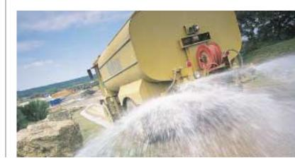
Whenever we're working our water trucks are out there, spraying water to control dust generated during mining activities. At many locations we also wash trucks before they leave the plant, and water down the roads around our facilities. Most plants are closed-loop, which means we supply and reuse our own water.
