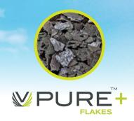
High purity vanadium flakes, mainly used in the production of master alloys. Approved by all master alloy producers around the globe.
